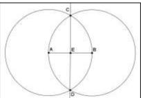
6 Construct circle BA, using point B as the center and point A as the endpoint
